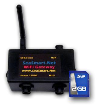
The SeaSmart.net<sup>™</sup> WiFi adapter can be used stand-alone to data log selected NMEA 2000 traffic to SD Memory or remotely accessed via the WiFi interface using TCP and UDP protocols supporting many devices over a single access point. When combined with a router with internet access or MiFi device, remote access to vessel NMEA 2000 data is possible anywhere, anytime.
