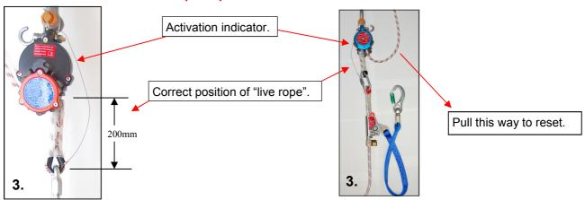
To reset the system, pull down on the dead end of the rope, see Pic 3, until the connection is within the accepted distance. The position of this connection must be monitored regularly and reset as required.
