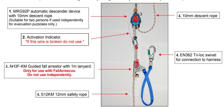
\*Always connect the AH3F to the 12mm S12KM safety rope\*
