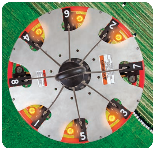
Bright LED lights show the pilot the number of the hook that is currently selected for release. In this picture, Hook 6 is armed for release. View gallery of light patterns at http://onboardsystems.com/carousel-light-gallery
