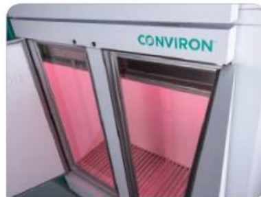
PG2500 Chamber with Valoya AP673 LED fixtures
