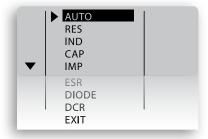
**AUTO MODE:** Select AUTO mode (AM sign appears at the left bottom corner of display) for automatic measurement of inductance, capacitance or resistance.
