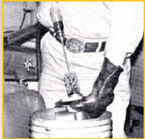
A smaller diameter Flex-Hone Tool is used in the finishing of master cylinders at RMP.
