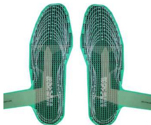
Figure A1-4: F-Scan in-shoe pressure sensors
