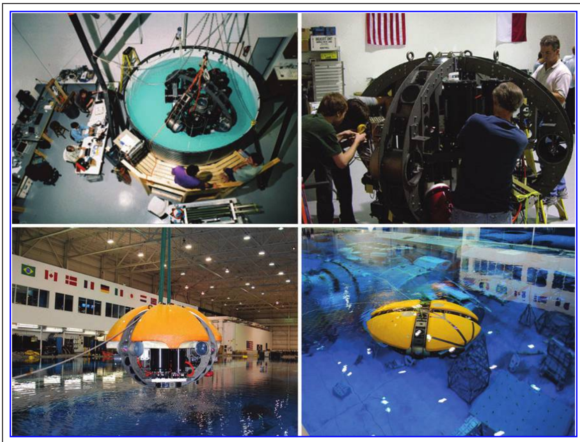
Fig. 6. Extensive engineering heritage. Top row: Design and construction of the fully autonomous Endurance extreme environment robotic vehicle as test prototype for NASA's Europa mission. Bottom row: Undergoing underwater testing at NASA's Neutral Buoyancy Facility at Johnson Space Center.
