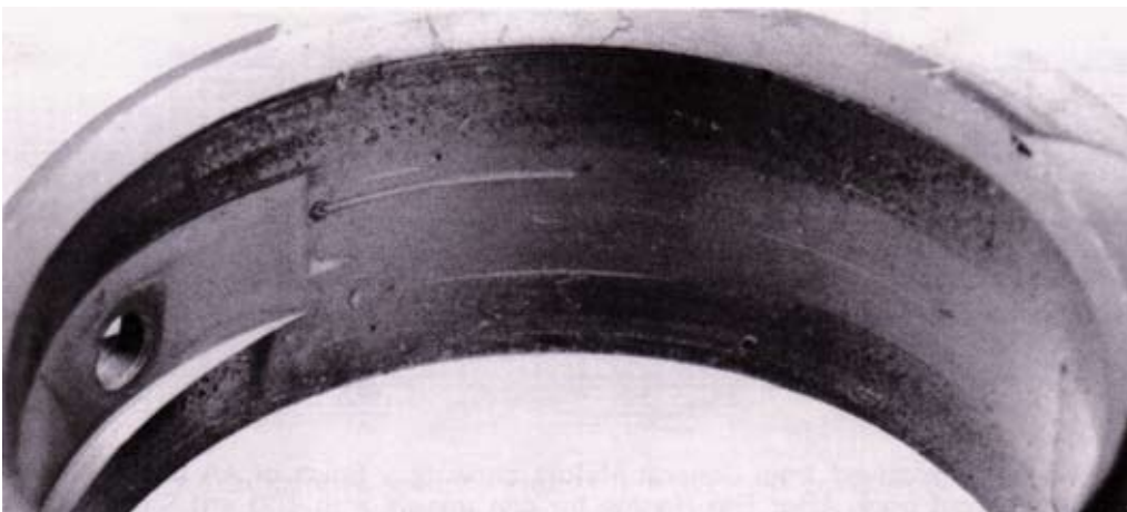
Bearing from No. 2 cylinder "A" engine after 24 hour run. An OEM new bearing such as were used in all the trials. Similar effects will be noted on all bearings as shown on the next page.
