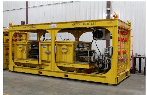
Figure 2 Battery-Powered Pump Skid at rest
