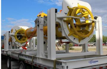
Figure 1 Static Mixer Module (SMM) installed within OceanWorks recently delivered Handling Aid ready for road transport.
