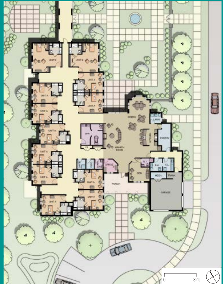
Several DFAR12 projects, like The Deupree House and Nursing Cottages, are reworking the layout of the Household for a better hierarchy of public-to-private spaces. Bedrooms no longer open into common areas, like living or dining rooms.
