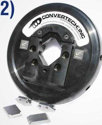
Quickly and easily replace inserts without removing the safety chuck.
