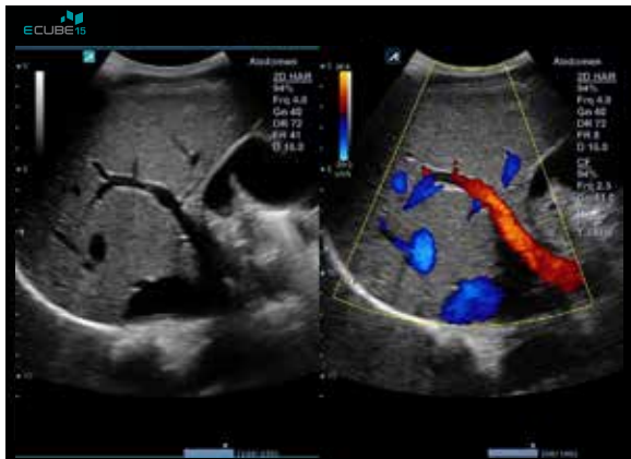
Tissue Harmonic Imaging(FTHI) of Liver in the Live Dual mode with Crystal Signature™ Transducer, SC1-4HS
