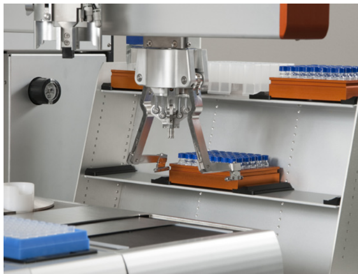
Figure 2: CM Protégé taking a plate from the integrated shoulder hotel to the balance.
