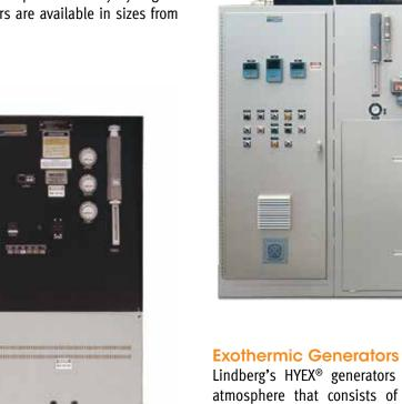
Lindberg's HYEX<sup>®</sup> generators provide a low cost protective atmosphere that consists of products of combustion. Air/ gas ratios can be varied to create a lean, non combustible atmosphere or a rich, combustible reducing atmosphere. These gas fired generators provide years of trouble-free operation. Sizes available from 500 to 15,000 cfh.
