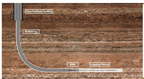
Through-the-bit technology allows the logging tools to pass through drill pipe and out of the drill bit, acquiring formation evaluation logs. These logs provide valuable, high-quality data that is used to make critical changes to drilling or completion designs and exploration targets. It's the type of data that is not possible to obtain with conventional logging technologies.
