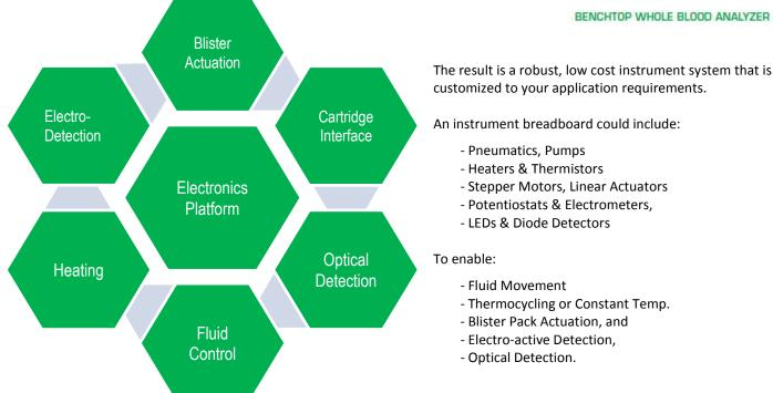
The Electronics Platform, or the brains of the instrument, ties all the sub-systems together with a user interface using a keyboard & monitor, or wirelessly with a tablet.
