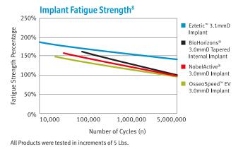
**Figure 1:** Endurance limits for narrow implants (n=11). Fatigue testing conducted per ISO 14801 demonstrated that at 5 million cycles Zimmer implants had an endurance limit that was 43% higher than that of Astra Tech, Nobel, and BioHorizons implants.
