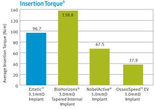
Benchtop engineering test utilizing a dense bone substrate.9
