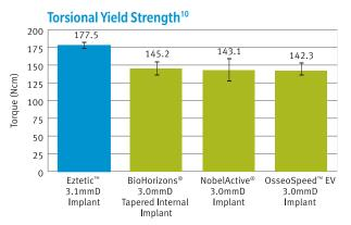
Benchtop engineering test utilizing the implants and their corresponding drivers.<sup>17</sup>
