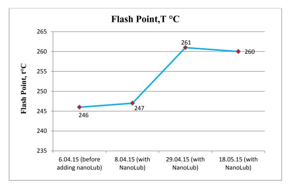
Flash point measurements demonstrate an improvement of thermal properties of the lubricant with about 16 °C increase.
