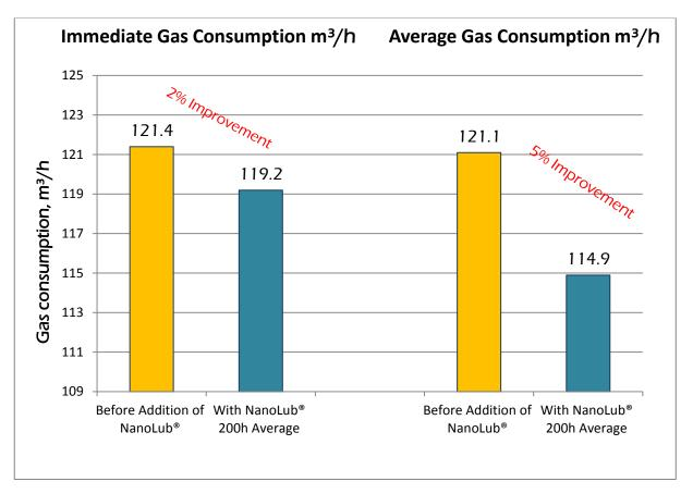
Immediate gas consumption was reduces by about 2%, while average gas consumption was reduced by about 5%, as measured by an average of 200 hours of work with 8 hour control periods.
