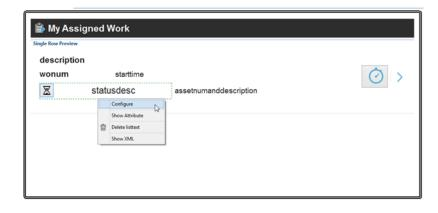
With Anywhere Builder, you can configure exact positioning of Maximo elements graphically, and see a live preview of the mobile device display while editing.
