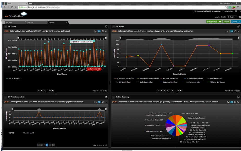
An example of using jKool to analyze and visualize Java Garbage Collection (GC) behavior). GC collections are analyzed across multiple JVMs with automatically computed upper and lower bands (normal bands). Bands auto-adjust, dynamically based on the incoming GC frequency and duration.
