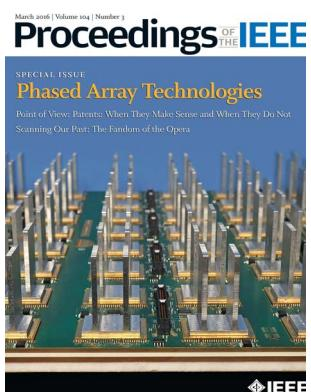
**On the Cover:** This month's cover photo features an electronic backplane of a Multipurpose Phased Array Radar panel for weather and air traffic control. The panel was constructed by applying modern low-cost manufacturing techniques for arrays. Photo Credit: MIT/Lincoln Laboratory.
