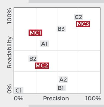
Metalcraft's RFID tags are consistently some of the best performing tags when tested for precision and readability. Precision measures for repeatability of the readings, while reliability measures the accuracy of the reading from varying distances, in different orientations. and on various materials.
