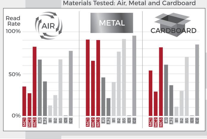
The most common material for Universal tags to be read on is metal, so that's the emphasis for performance during tag development. This study also shows how these on/off metal tags read on other common surfaces.
