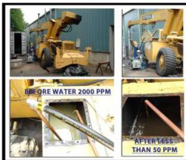
HYDRAULIC CRANE RESERVOIR CONTAMINATED WITH 2000 PPM WATER
