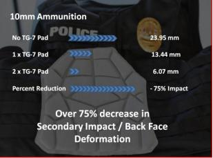
»The patented TG-7 Ballistic Armor Protection Inserts are designed to be worn underneath Ballistic Vests. The TG-7 and TG-7U, when worn beneath current soft armor vests, provide extra protection against trauma from back force deformation from bullet strikes, reducing additional injuries.
