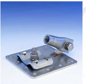
APPLICATION: This is the most universal base in the industry. The swivel adaptor allows the air terminal to level under most conditions. It can be secured with screws, nails, ¼"bolts, ¼"drive-in anchors, or an adhesive. Bolt tension cap can be turned so the cable can run horizontal of vertical. Perfect for any uneven surface. Furnished for all air terminal sizes 3/8", ½", or 5/8", specify when ordering.
