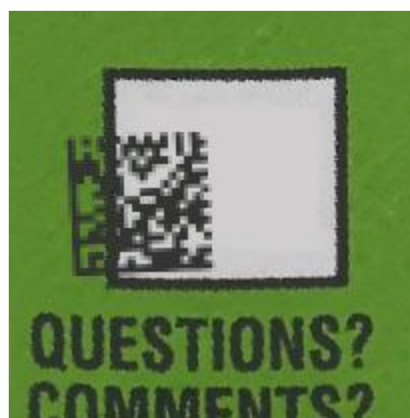
Insufficient quiet zone
