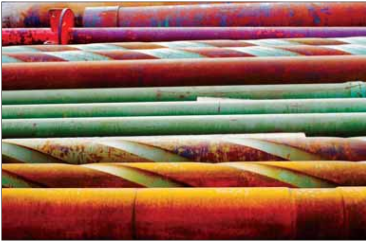
1st Place: Drill Casings for New Geothermal Well by Cari Covell, Reykjavik University - Iceland School of Energy, Reykjavik, Iceland
