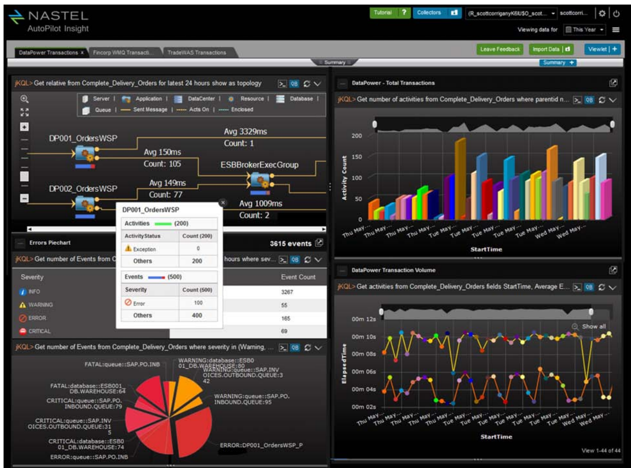
Figure 12: An example of an AutoPilot Insight dashboard with application topology showing transactions spanning Web Apps, IBM DataPower and an ESB
