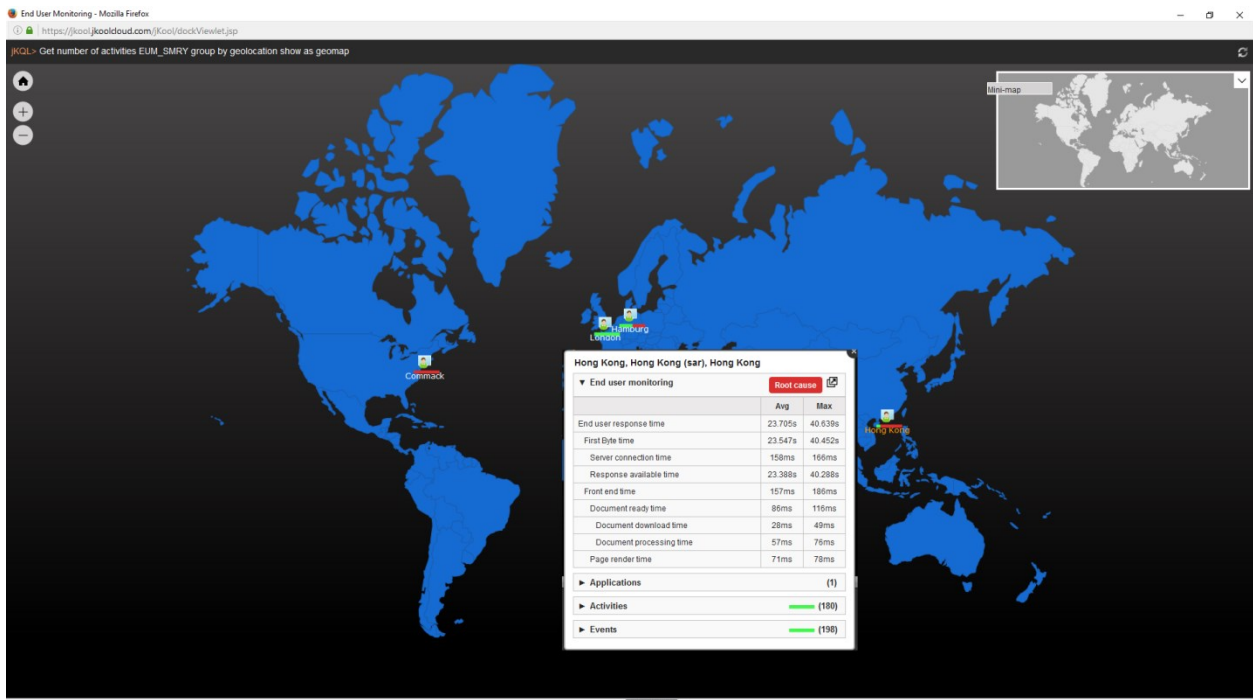
Figure 9: Real-User Monitoring provides analysis of end-user experience using injection-based, browser instrumentation. The request from the browser is broken up into all its components and measured for latency. The user transaction is stitched to back-end server transactions. The root cause button will take the user to the probable root cause of the latency the end-user is experiencing.
