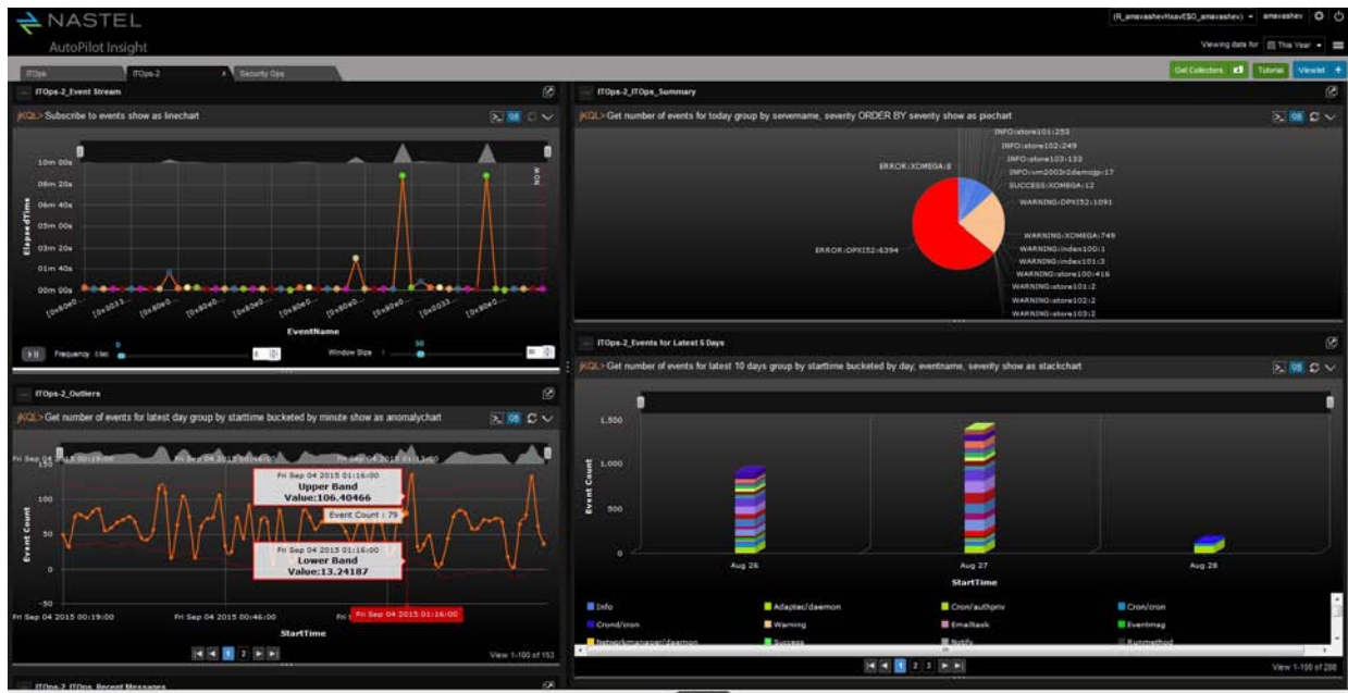
Figure 1: An example of an operational intelligence dashboard. The data displayed is streaming into AutoPilot Insight from Log4j and Syslog Collectors.
