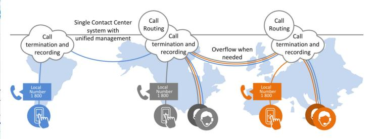
Figure 4: Global contact center operation using a single cloud contact center vendor with multi-tenants and multi-clouds
