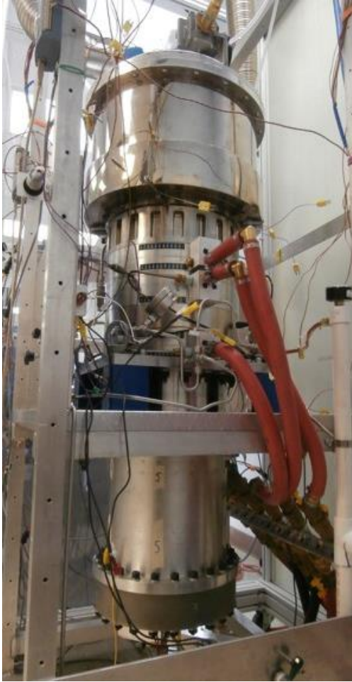
2 nd -Generation TC-Cycle™ prototype in test cell which has reached operational temperatures as low as -10°C
