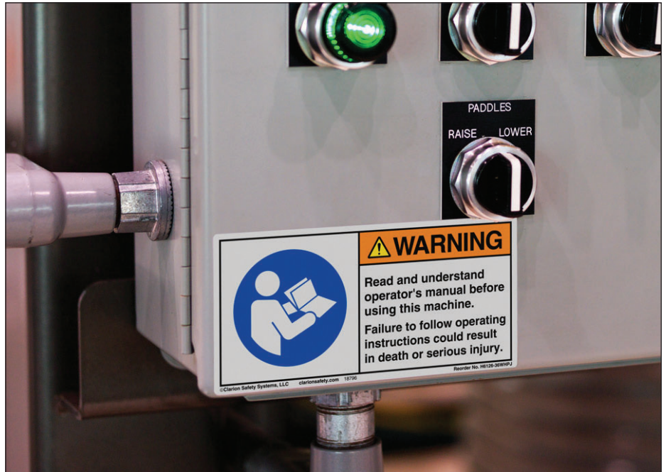
Figure 2: A best practice ANSI Z535 safety label, including the ISO 7010 safety symbol for "refer to instruction manual/booklet" (©Clarion Safety Systems. All rights reserved.)
