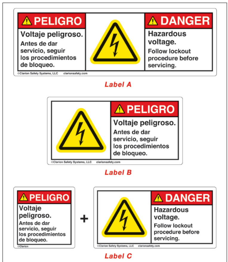
Figure 1: Safety label formatting options using additional languages can include multilingual labels (Label A), foreign language labels (Label B), or add-on foreign language labels (Label C). (Label designs ©Clarion Safety Systems. All rights reserved.)
