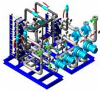
<Hot water + Hot tap water (2stage)>
