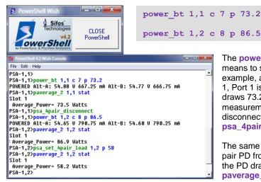
Class 7 4-Pair Power-Up and Shutdown on Port 1 followed by Class 8 Power-Up on Port 2
