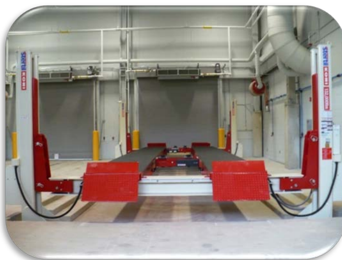
Massive Stertil-Koni 4-post lift, ST 4600, delivers optimal high-capacity lifting for oversized vehicles
