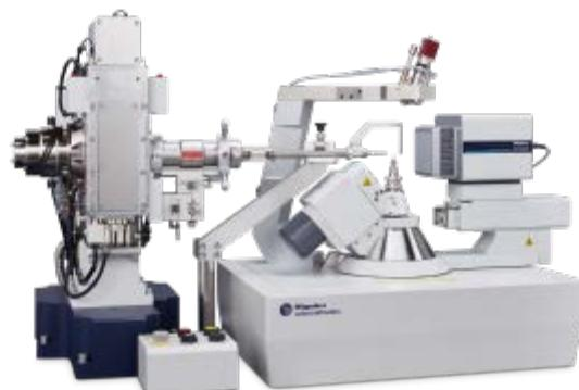
Rigaku XtaLAB Synergy-Custom X-ray diffraction system
