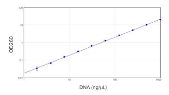
The SpectraMax iD5 reader is fully compatible with the SpectraDrop Micro-Volume Microplate, enabling quantitation of precious low-volume samples. 4- $\mu$ L DNA standards from 2 ng/ $\mu$ L to 1000 ng/ $\mu$ L were read in absorbance detection mode with a preconfigured protocol in SoftMax Pro Software. Performance matching the 2 ng/ $\mu$ L sensitivity specification is demonstrated here.
