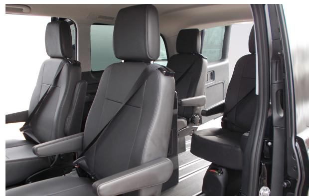
The TransitWorks Metris Business Line comes with a custom engineered fold-out center-aisle table and integrated storage compartment. Forward facing seats on our exclusive floor track are quickly transformed into a functional work space.
