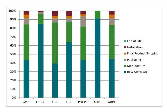
Figure 4: VDS Lite by Forster Framing System Environmental Impact Potentials (CML 4.1)
