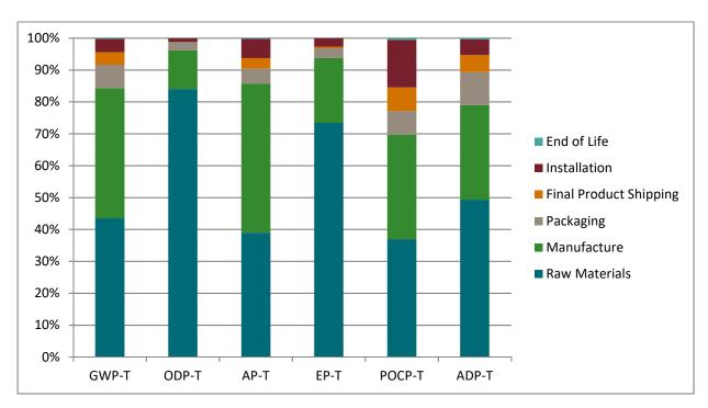
Figure 3: VDS Lite by Forster Framing System Environmental Impact Potentials (TRACI 2.1)
