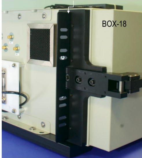
Rack-mounting brackets for a 19" rack
