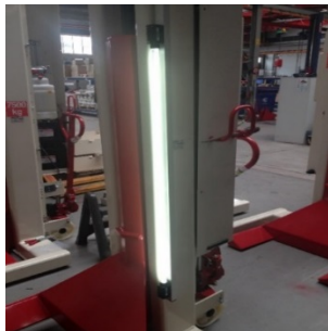
Consisting of two IP-67 rated fixtures, illumination is available on all mobile lifts manufactured by Stertil-Koni
