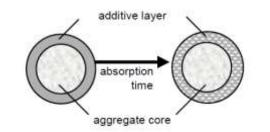
Figure 1. Configuration of Remind-coated particle.
