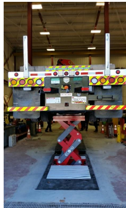
The scissor-style ECOLIFT allows for wheels-free lifting
