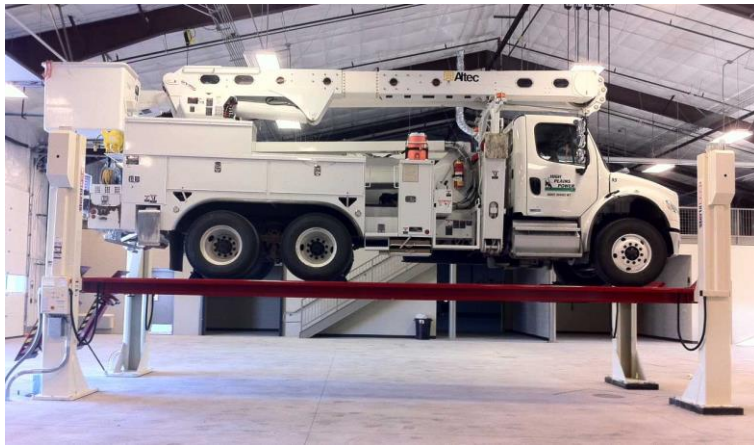
A utility company from the western United States utilizes the Stertil-Koni 4-post lift when servicing this bucket truck
