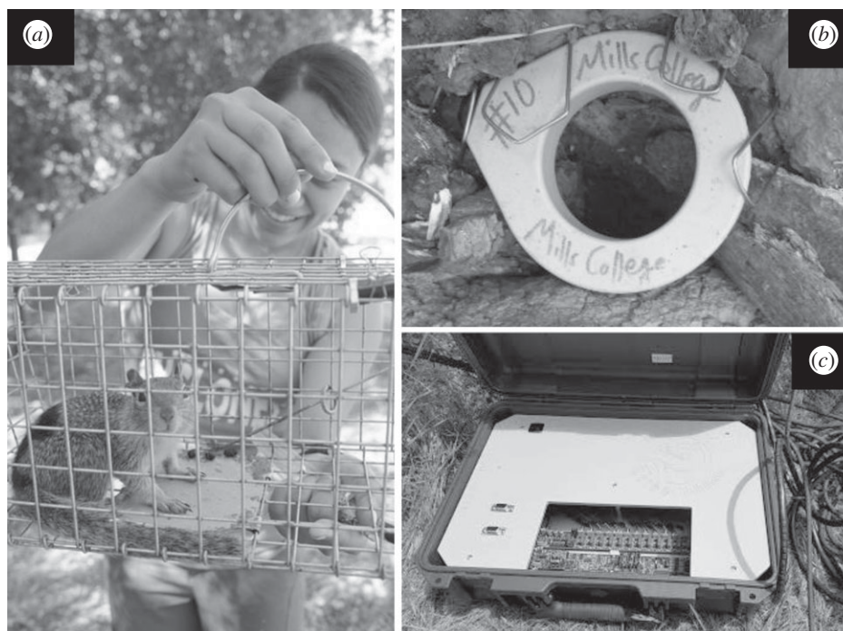
Figure 1. Novel automated-tracking system. (a) Live trapping and release of free-living California ground squirrels allow researchers to provide each individual with a unique fur mark for visual identification during social observations, ear tag for identification during trapping and passive integrated transponder (PIT) tag beneath the skin for detection by the monitoring system. (b) Movements are detected by scanning an individual's PIT tag every time it passed through a secure antenna loop inside of a burrow opening. (c) Data logger (Biomark, Inc., Boise Idaho) records information about the time of day, squirrels' PIT tag ID and burrow location for each movement event. (Online version in colour.)
