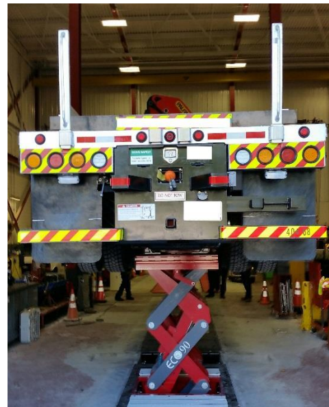
ECOLIFT is available in both a 2-scissor or 3-scissor configuration; total lifting capacity is 60,000 lbs. and 90,000 lbs. respectively – at 30,000 lbs. per scissor.
