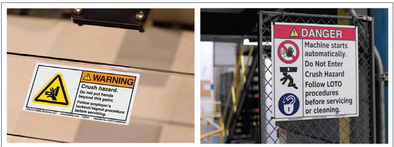
Figure 2: A product safety label placed on a guard on a piece of equipment (at left) and a safety sign warning of automatic startup on a machine in a facility (at right) (Label and sign designs ©Clarion Safety Systems).
