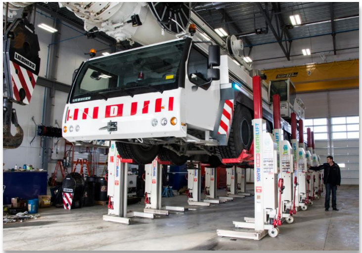
Wireless mobile column lifts are efficient, safe, portable and minimize operator tripping hazards as there are no interconnecting communications cables
