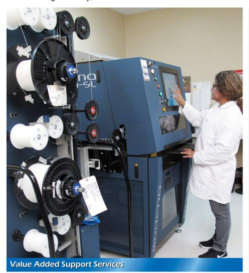
As a cost effective solution, CIA&D (Co-Operative Industries Aerospace & Defense) provides marking services for customer supplied materials. With state-of-the-art laser identification technology, CIA&D can permanently mark a broad range of wire and cable jacket types and constructions to meet customer specific requirements.
