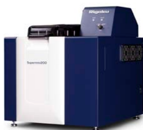
Rigaku Supermini200 wavelength dispersive X-ray fluorescence spectrometer
